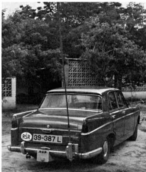
Helically wound mobile whip for 10-80 meters used by ZE6JP.
